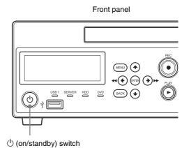
When the unit turns on, the front panel display lights and "WELCOME" appears.
