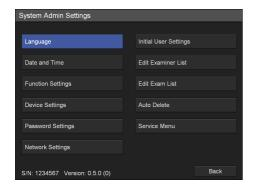
The setting screen for the selected item appears. The serial number of the unit and the current software version appear at the bottom left.
