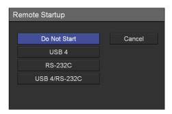
When [USB 4] or [RS-232C] is selected, the remote system's on/off operation will be linked to that of the unit via the selected connector.
