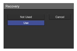
Recovery of recorded data is the only action performed when [Not Used] is selected.
